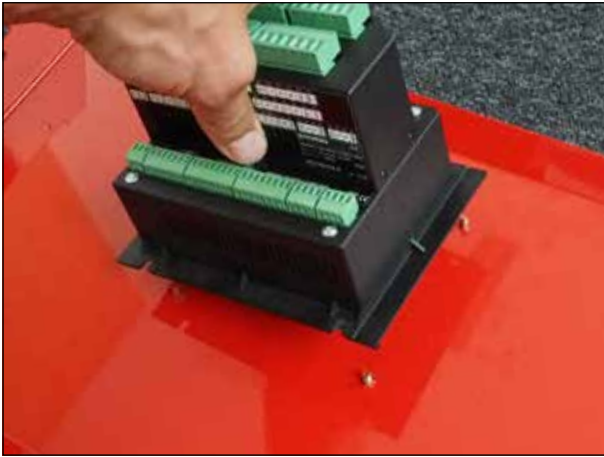
Installation of the controller on four M4 screws
